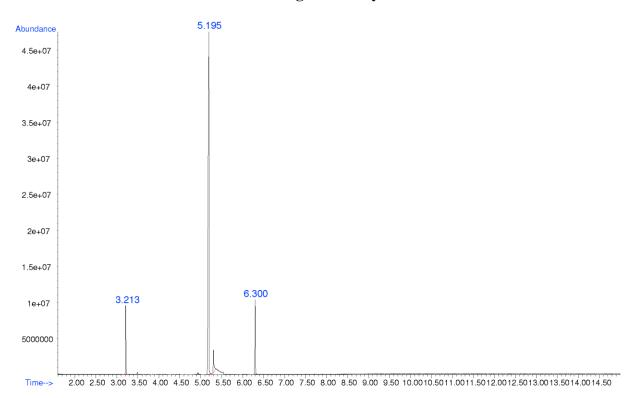
Additional peaks present in chromatogram: internal standard 1 (3.213 min), internal standard 2 (6.300 min)
