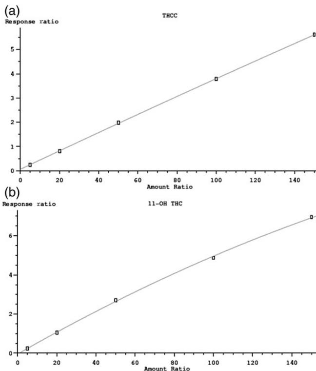
Figure 2. Examples of calibration curves for (a) THCC and (b) 11-OH-THC.
